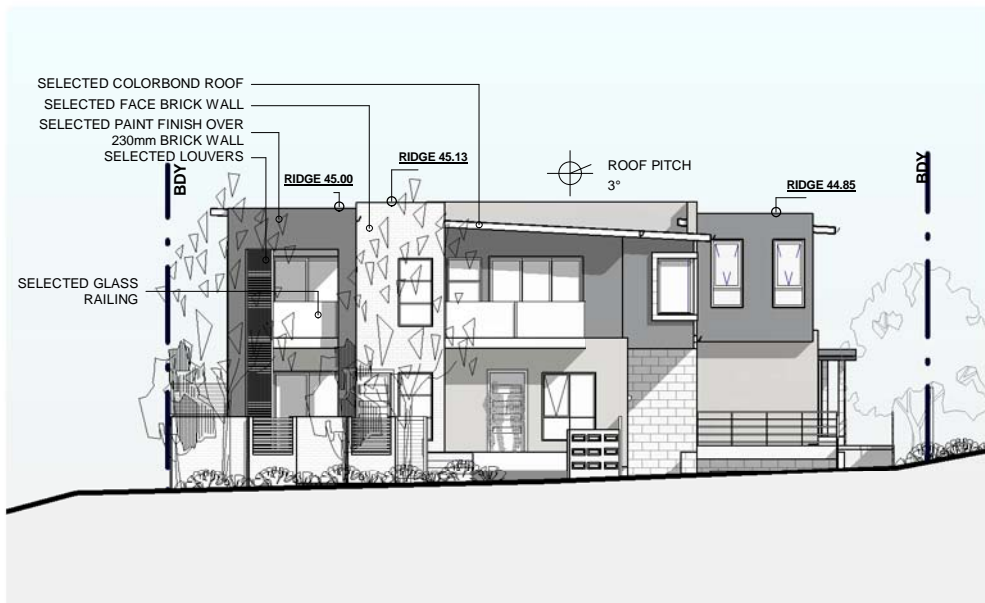
1 FRONT ELEVATION- NORTH DA300 1 : 200
